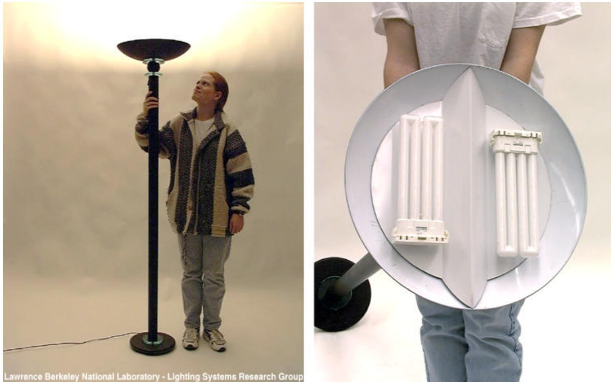
*Figure 1: An example of a CFL Torchierie based on LBNL prototypes that is now available in the marketplace. The luminaires are similar in look to halogen torchieres, but they use two fluorescent lamps in a white reflector dish (as seen on right).*
