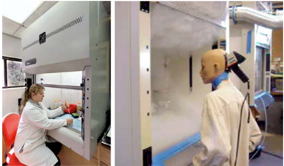
Fig. 10 Prototype high-performance fume hood. Air is introduced in the frame (face) of the hood, in front of the worker (see grill under right wrist), maintaining or improving containment and reducing energy use. Typical designs draw air from the general lab space around the worker, causing turbulence and higher-than-necessary fan energy use. Smoke in right panel shows air entering through the frame
