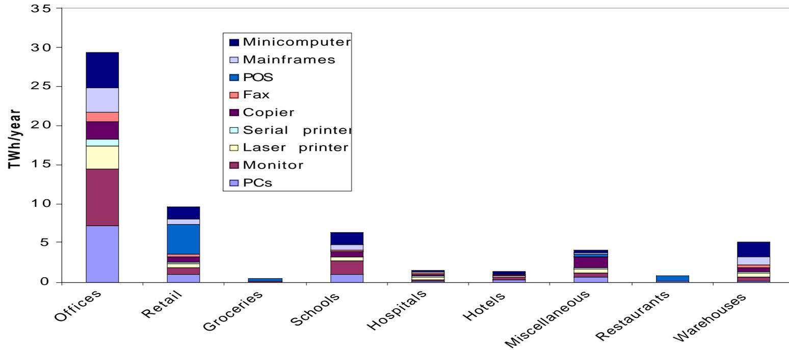
**Figure 3.2: Commercial-sector U.S. office equipment electricity by equipment type and building type**
