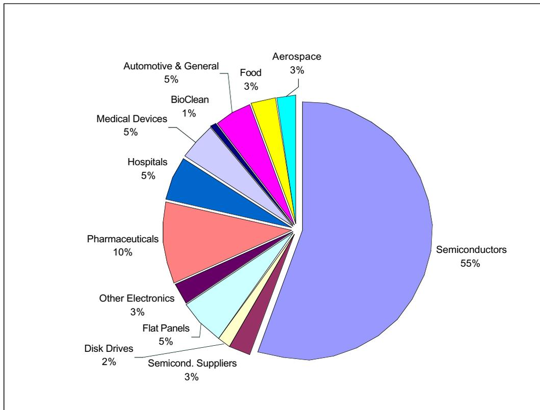
**Figure 5-2: Share of HVAC Electricity Consumption for Cleanrooms**
