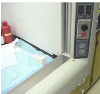
Figure 15. Lower supply grill detail.
