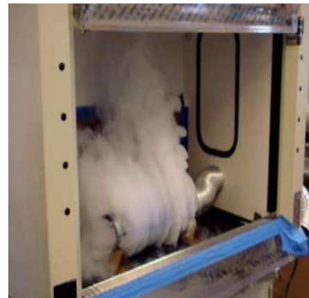
Figure 4. Berkeley Hood, showing full containment during flow-visualization test.
