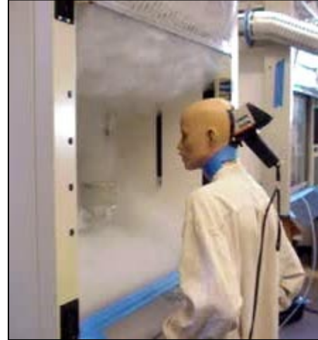
Figure 3. Berkeley Hood, showing patented air-divider supply effect.
