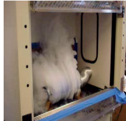
Figure ES-4. High-performance Berkeley Hood, showing full pollutant containment during flow-visualization test.
