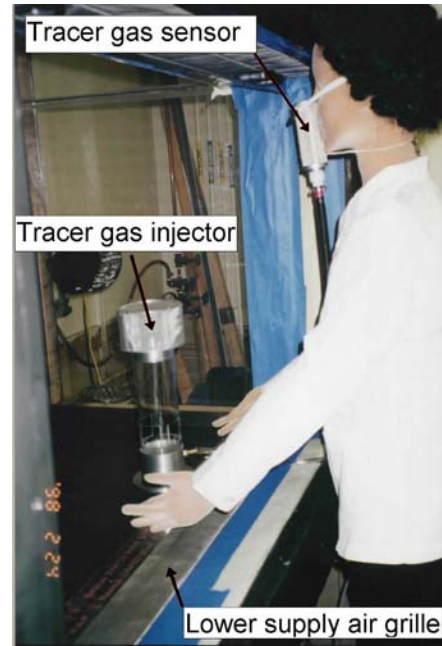
Figure 5. Setup for tracer gas test, with injector and mannequin in “right” position.
