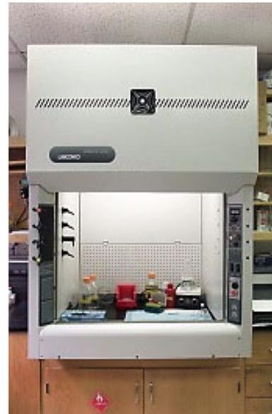
**Figure ES-5. Labconco alpha prototype Berkeley Hood.**
