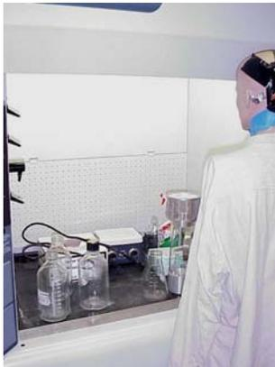
**Figure 20. Hood with clutter, left view.**
