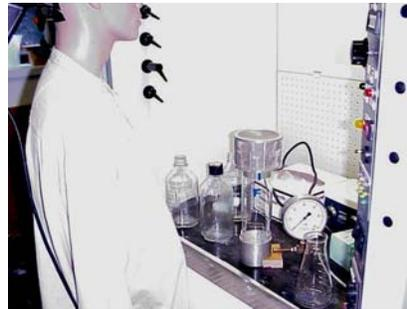
**Figure 21. Hood with clutter, detail.**
