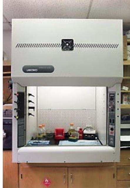
*Figure 7. Labconco alpha prototype Berkeley Hood.*
