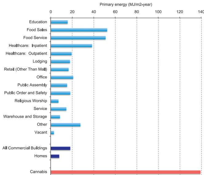
Fig. 4. Comparative energy intensities, by U.S. building type (2003).
