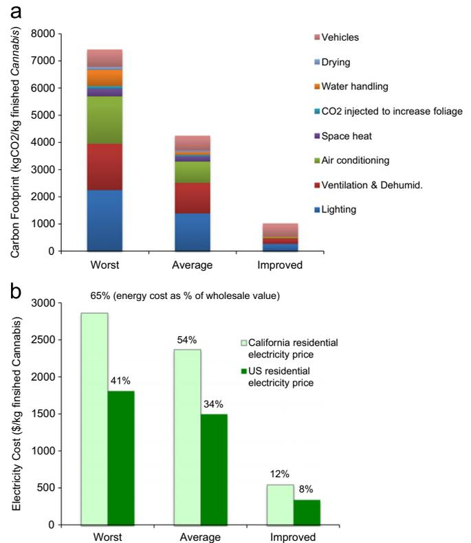
**Fig. 2.** Carbon footprint and energy cost for three levels of efficiency. (a) Indoor cannabis: carbon footprint. (b) Indoor cannabis: electricity cost. Assumes a wholesale price of \$4400/kg. Wholesale prices are highly variable and poorly documented.
