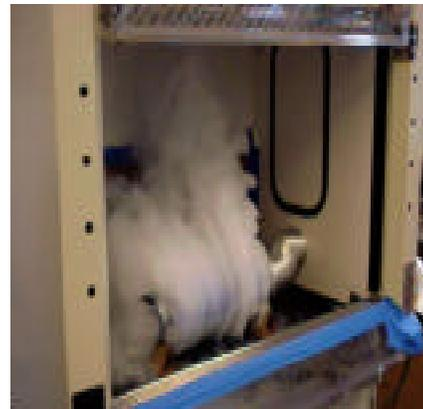
**Figure 11. Berkeley Hood, showing full containment.**
