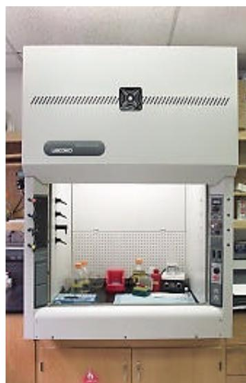
**Figure ES-5. Labconco alpha prototype Berkeley Hood.**
