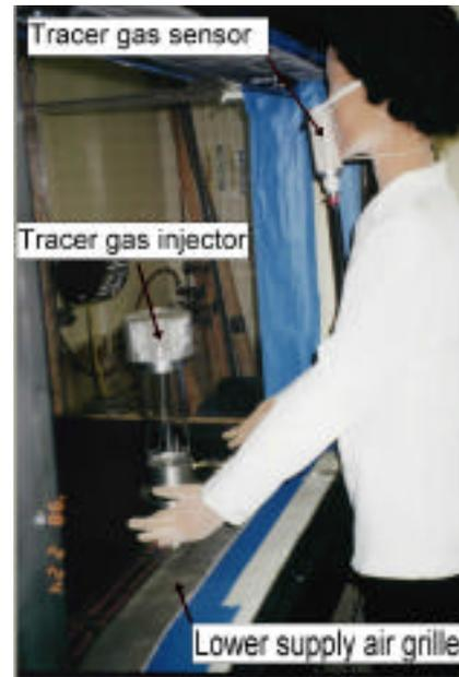
**Figure 12. Setup for tracer gas test, with injector and mannequin in "right" position.**
