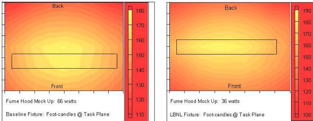
**Figure 9. Iso-lux plots at work plane: standard fume hood lighting and Berkeley Hood. The resulting pattern of illumination is more uniform (less of a range in light levels, measured in footcandles) and more well-centered over the work area.**
