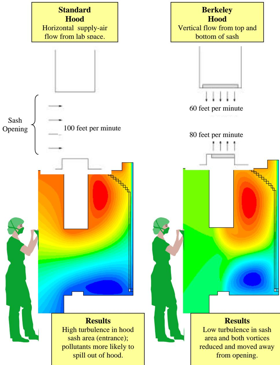
Researchers completed modeling on both a generic design and an actual fume hood superstructure. Initial CFD runs were computed prior to LBNL obtaining an actual fume hood superstructure from our industrial partner. Therefore, geometric relationships were generalized with respect to sash size, interior dimensions, back-baffle arrangement, etc. These runs varied air flow quantities for all three supply plenums and overall exhaust quantity.
