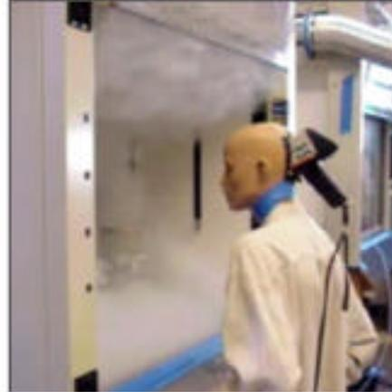
**Figure 10. Berkeley Hood, showing airflow pattern from sash-integrated air supply.**
